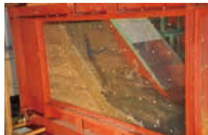
斜面崩壊後 The slope model after the test. The model failure
