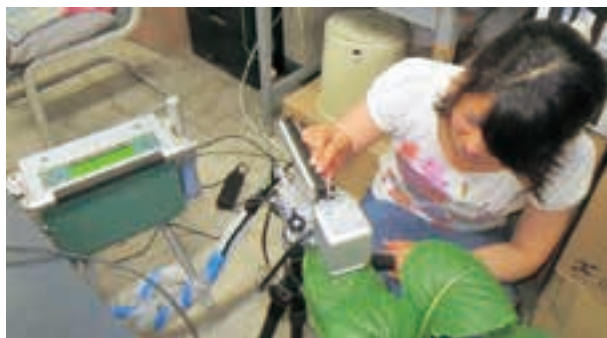
農作物の純光合成速度と蒸散速度の測定 Measurements of net photosynthetic rate and transpiration rate of crop plants
